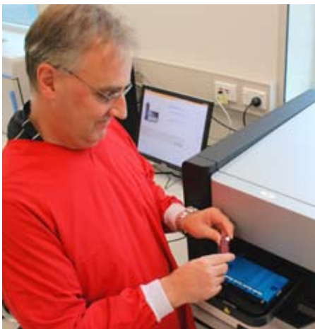
AgResearch Senior Scientist John McEwan loading a new Illumina Ovine SNP50 BeadChip onto the machine that measures results. Scoring more than 50,000 genetic variations at once, the chip will enable farmers to breed better sheep, faster.
